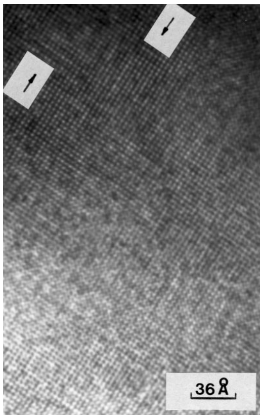
FIG. 3. The high-resolution lattice image in [100]_c projection. The arrows indicate weak contrast features in the form of rows of brighter and darker lines spaced by a_c and 10–20 unit cells long (40–80 Å) in the thicker parts of the fragment.
